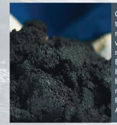
Oil sands, sometimes referred to as tar sands, are naturally occurring mixtures of bitumen, sand, water, small amounts of heavy metals and other contaminants. Each grain of sand is surrounded by a layer of water and a film of bitumen. The oil sands are found mainly in the Athabasca, Peace River and Cold Lake areas of Alberta.
